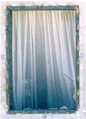
Pre- and Post-test exterior views of the window protected with the Safetydrape® blast curtain system.
