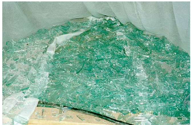
Pre- and Post-test exterior views of the window protected with the Safetydrape® blast curtain system.
